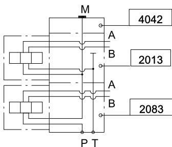
8.2.4 Series circuit - Circuit with more than three solenoid valves
