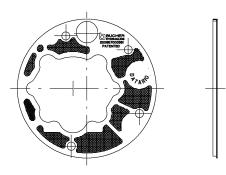
Filter conveyor PATENTED Assembled on the return line Plastic material Polyester filter area 150 micron filtering net Fixed directly on the housing Seal for the pump body.
