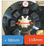
Large die opening = no need to remove dies Radial die travel = easy positioning of fitting
