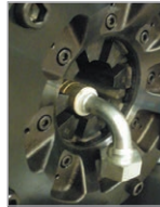
Front flange cuts allow long drop elbows
